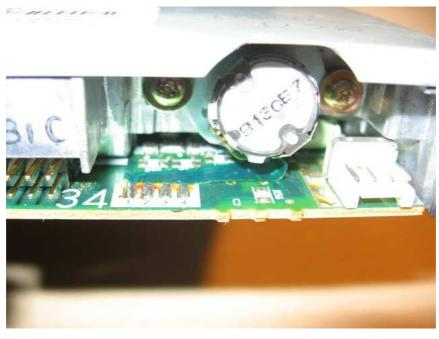
• Set ds to ds0, ry/dc to ry and solder a jumper from the ry/dc switch dc pad to pin 2 on the floppy connector (edgemost pin)
